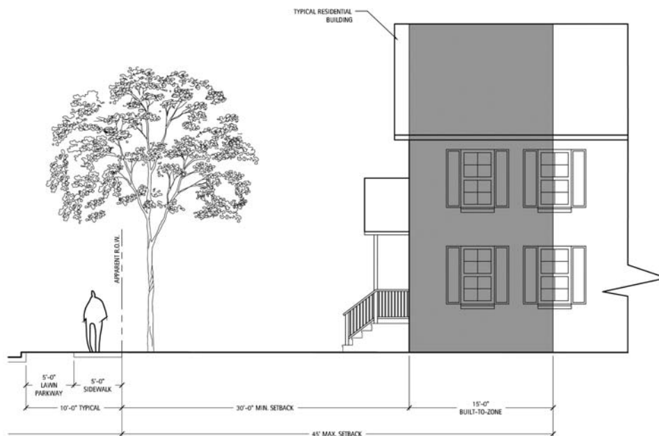
Figure 3.24: Typical Section in MT District
