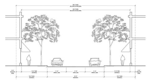
Figure 3.15: Section of Typical Toft Avenue Roadway Section in TC District
