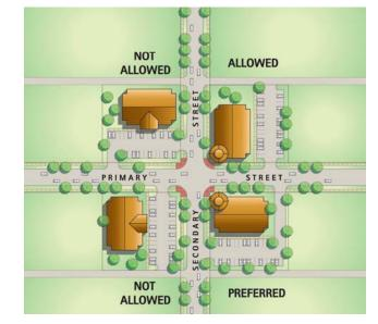
Figure 3.10: Building Massing/Parking location requirements
