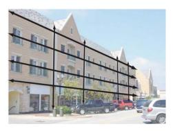
Building design should feature a balance of vertical and horizontal elements, as illustrated by the lines on the above photograph.
