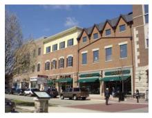
Facades "broken up" with articulation and roofline changes to create a "built over time" appearance.
