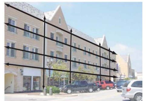
Building design should feature a balance of vertical and horizontal elements, as illustrated by the lines on the above photograph.
