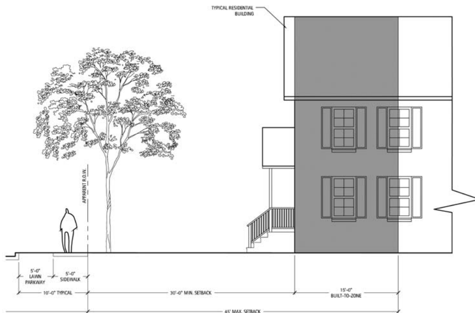
Figure 3.24: Typical Section in MT District
