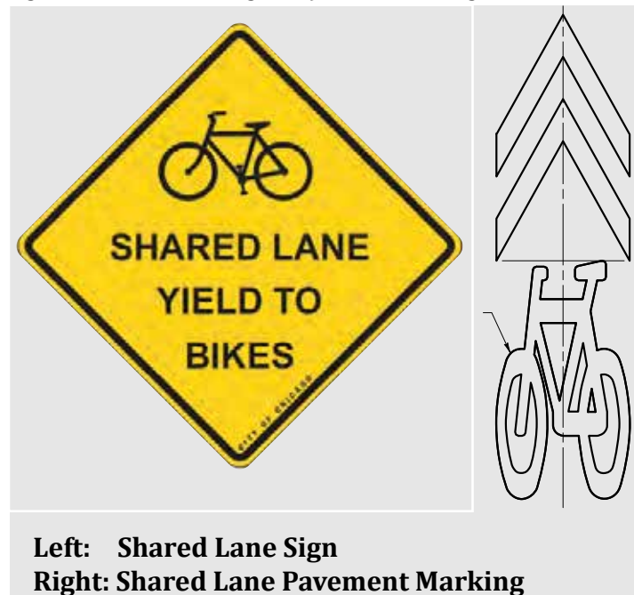
Figure 4.24. Shared lane sign and pavement markings
