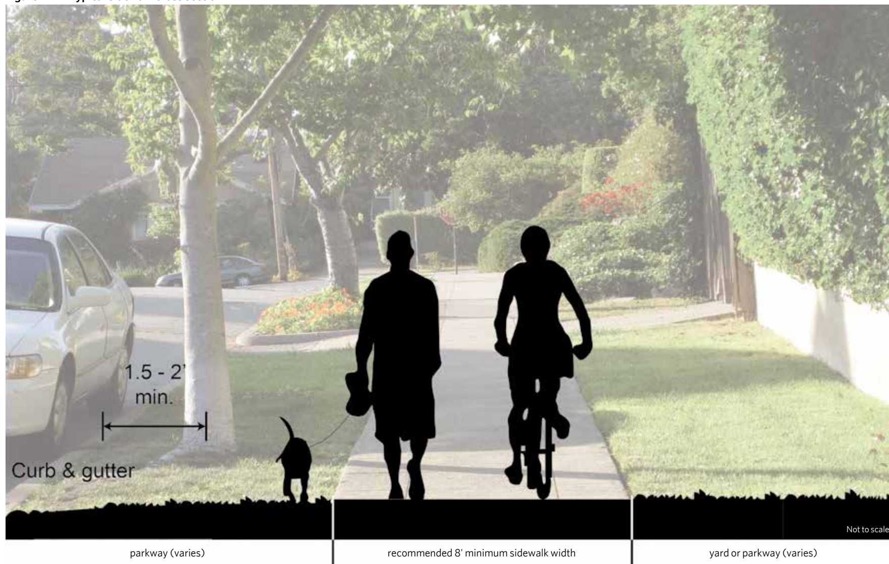
Figure 4.22. Typical sidewalk cross section
