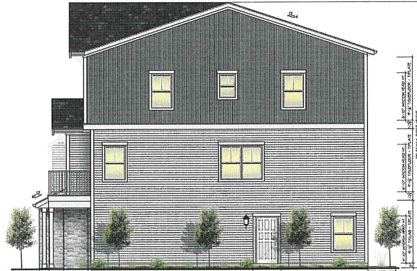
BUILDINGS 2-7 - A UNITS RIGHT ELEVATION 1/4" = 1' 0"
